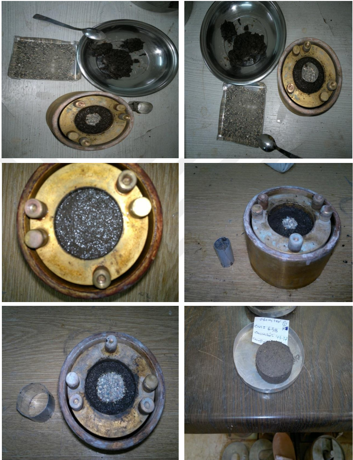
Figure 3.8: Steps for sample preparation for consolidation test
