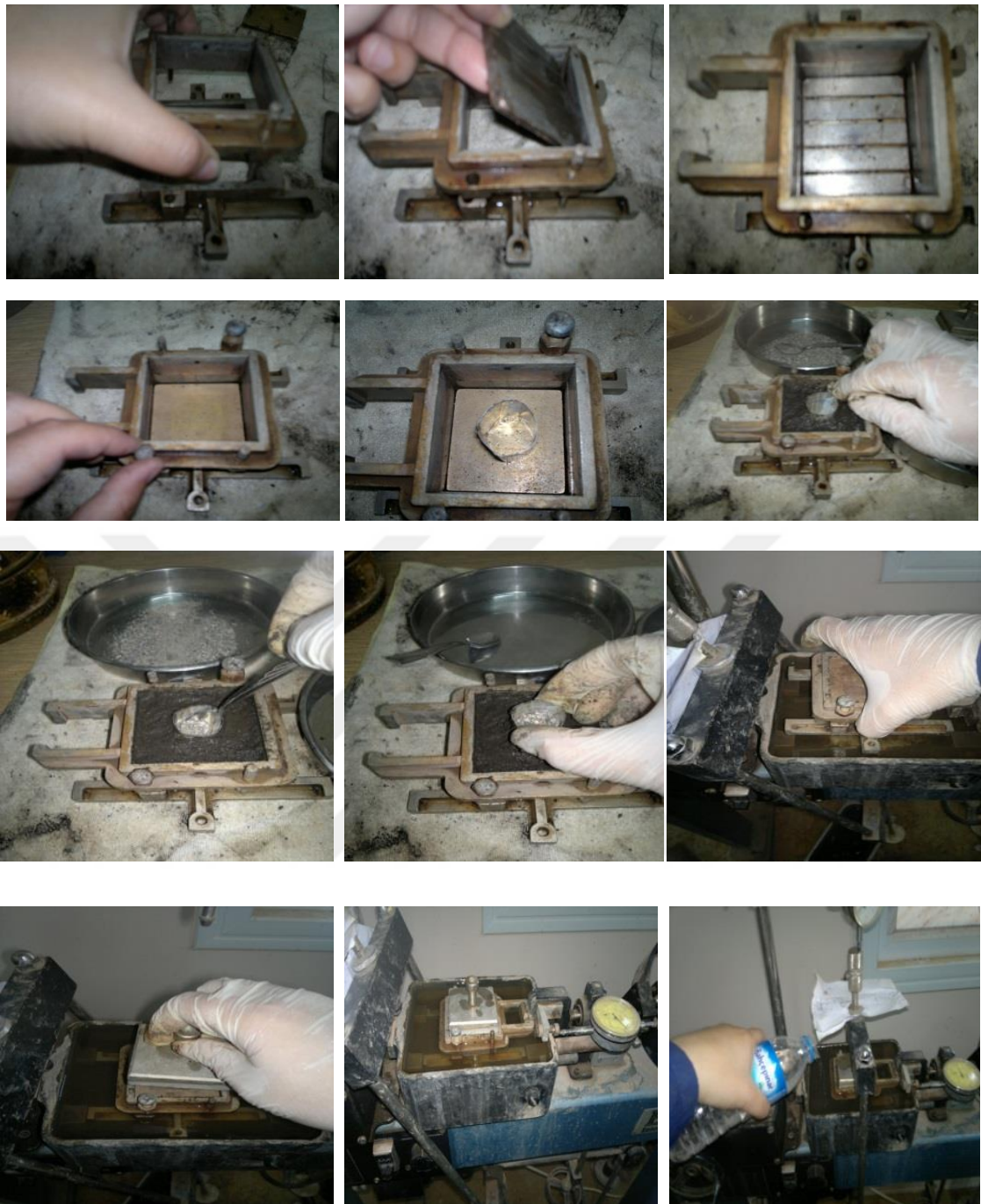
Figure 3.10: All procedures of direct shear test
