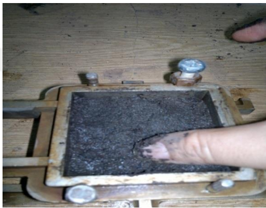
C21: Preparing samples for direct shear test
