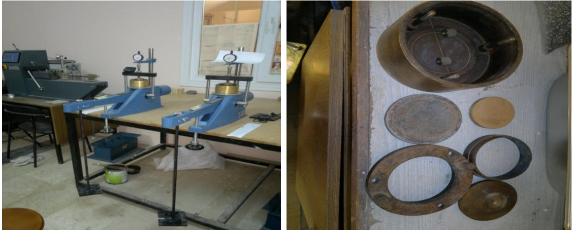
Figure 3.7: Standard consolidation assembly of all components of Oedometer test
