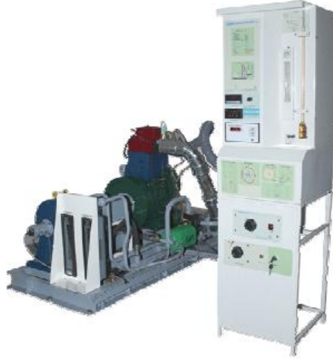
Figure 3.1. VCR spark ignited engine test rig
