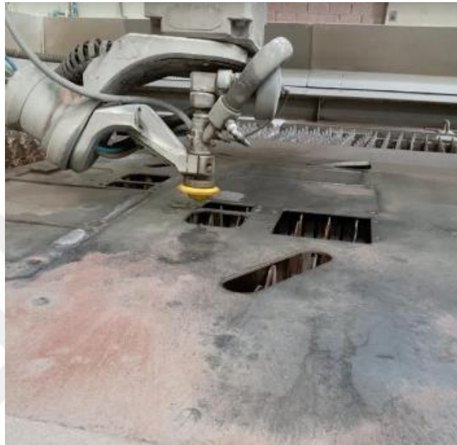
Figure 4.8. Steel Cutting Process with Waterjet
