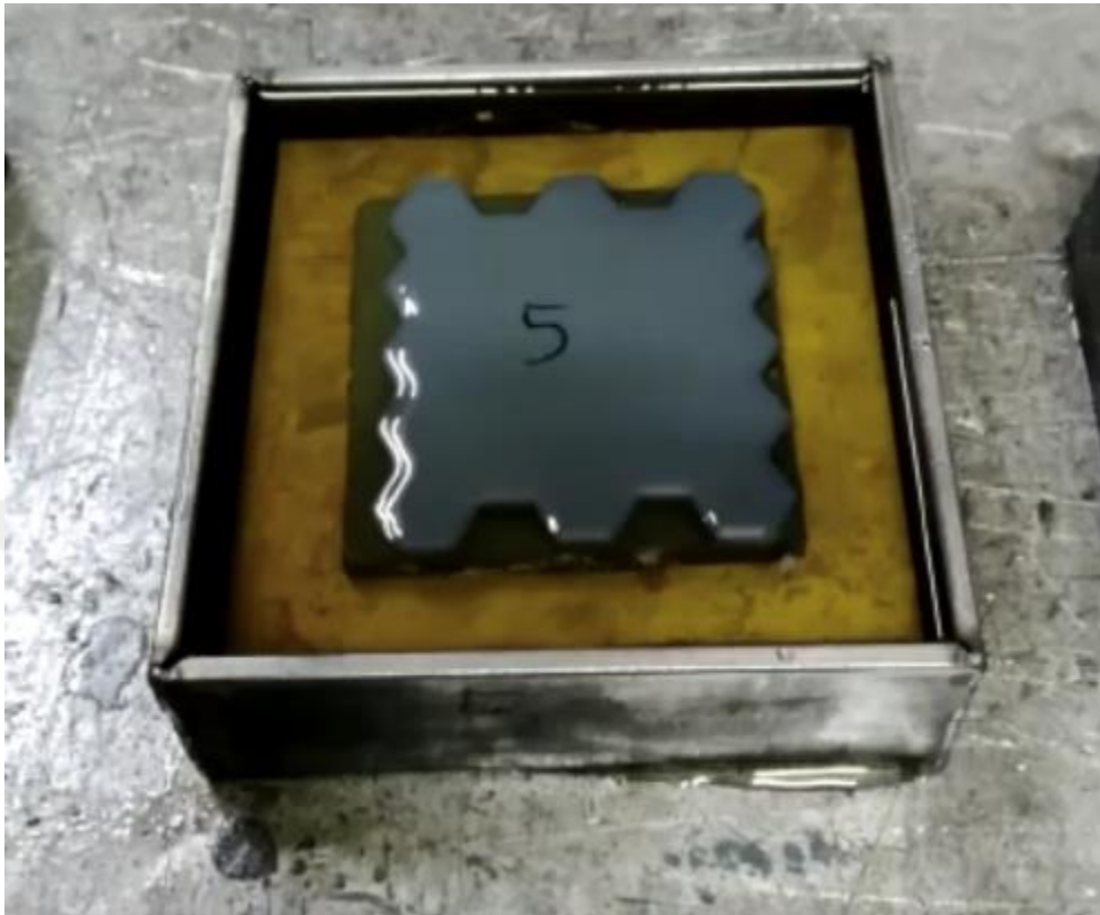
Figure 4.12. Epoxy Resin Application to Ceramic Tiles
