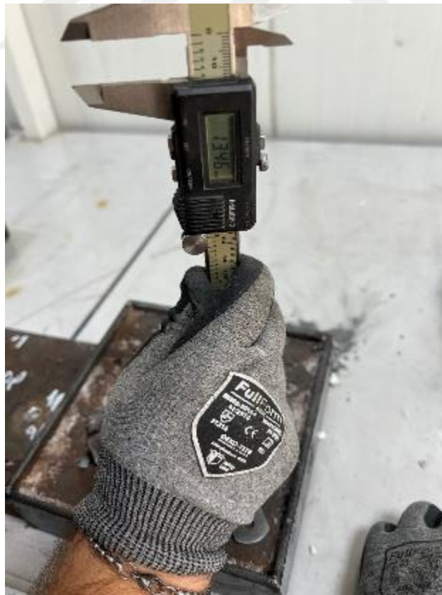
Figure 4.29. Depth of Penetration on Configuration – 3 After First Impact (13,46 mm from surface)
