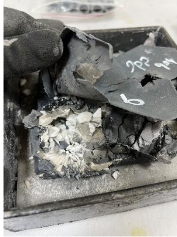
Figure 4.32. Broken Ceramic Tiles of Configuration – 4 after Ballistic Impact
