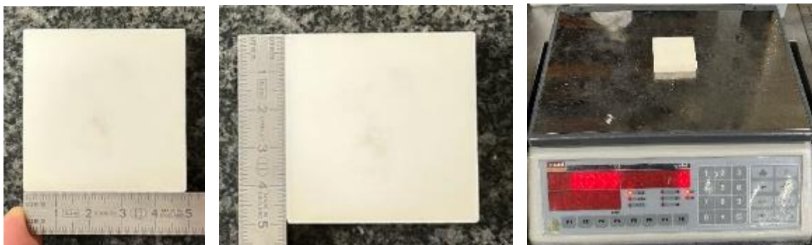
Figure 4.16. Dimensions and Mass of the Alumina Tiles
