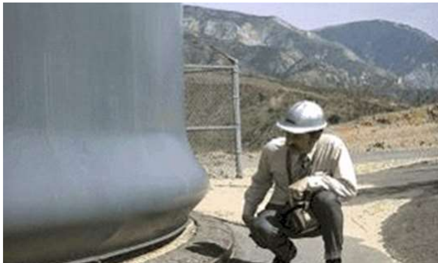
Figure 2.2 Elephant foot buckling [43]
