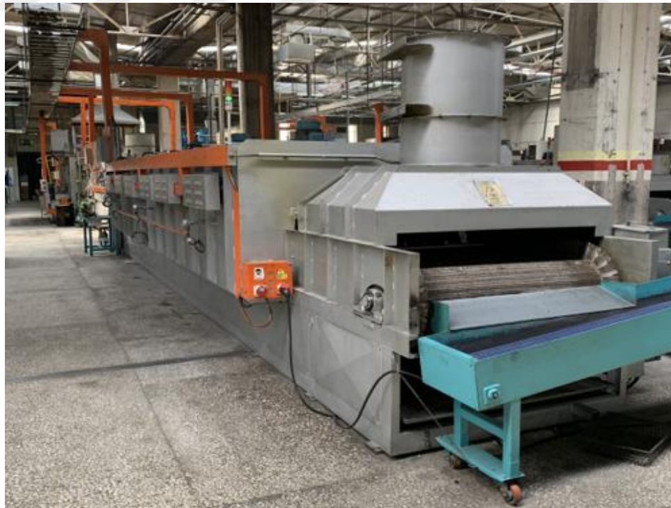
Figure 2.6 Aichelin tempering furnace for both types of rings
