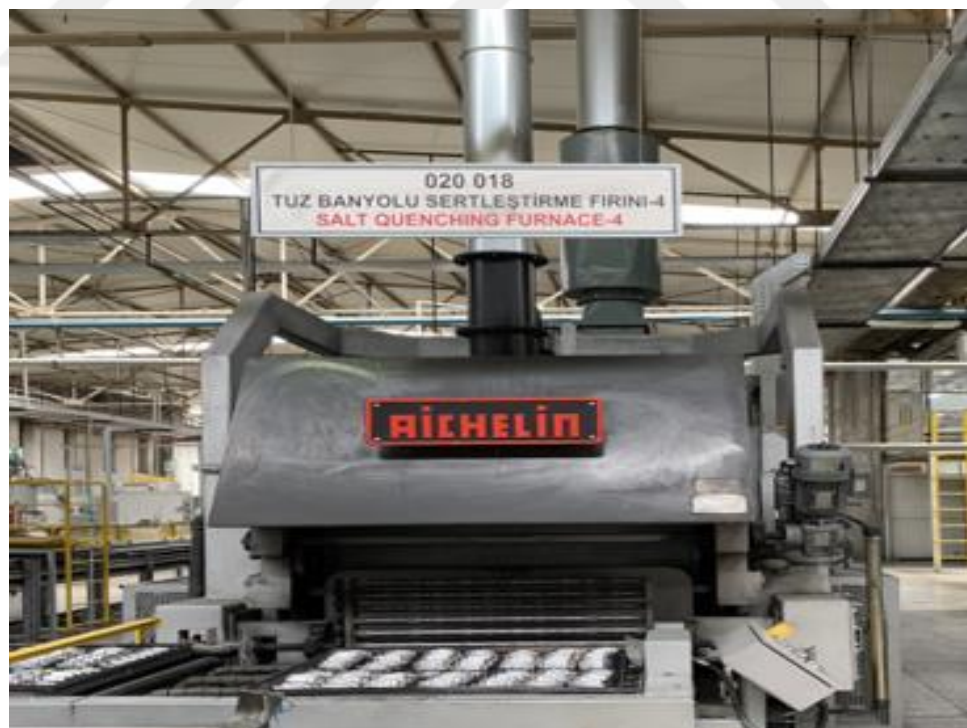
Figure 2.5 Salt Quenching Furnace (20 018) for through hardening of outer rings
