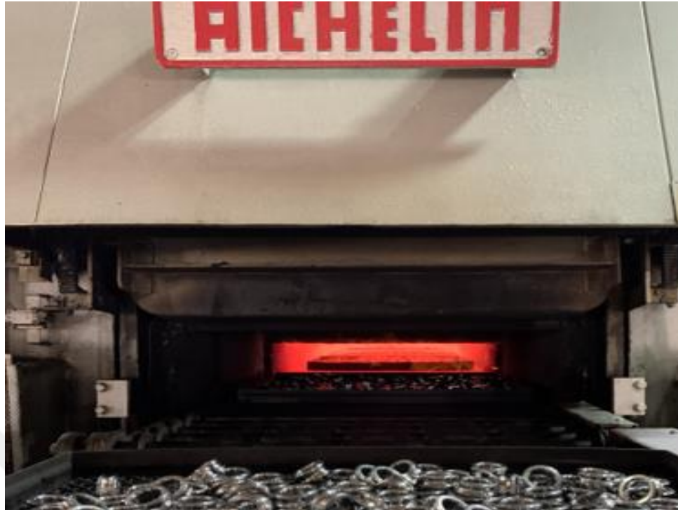
Figure 2.4 Oil Quenching Furnace (20 014) for through hardening of inner rings
