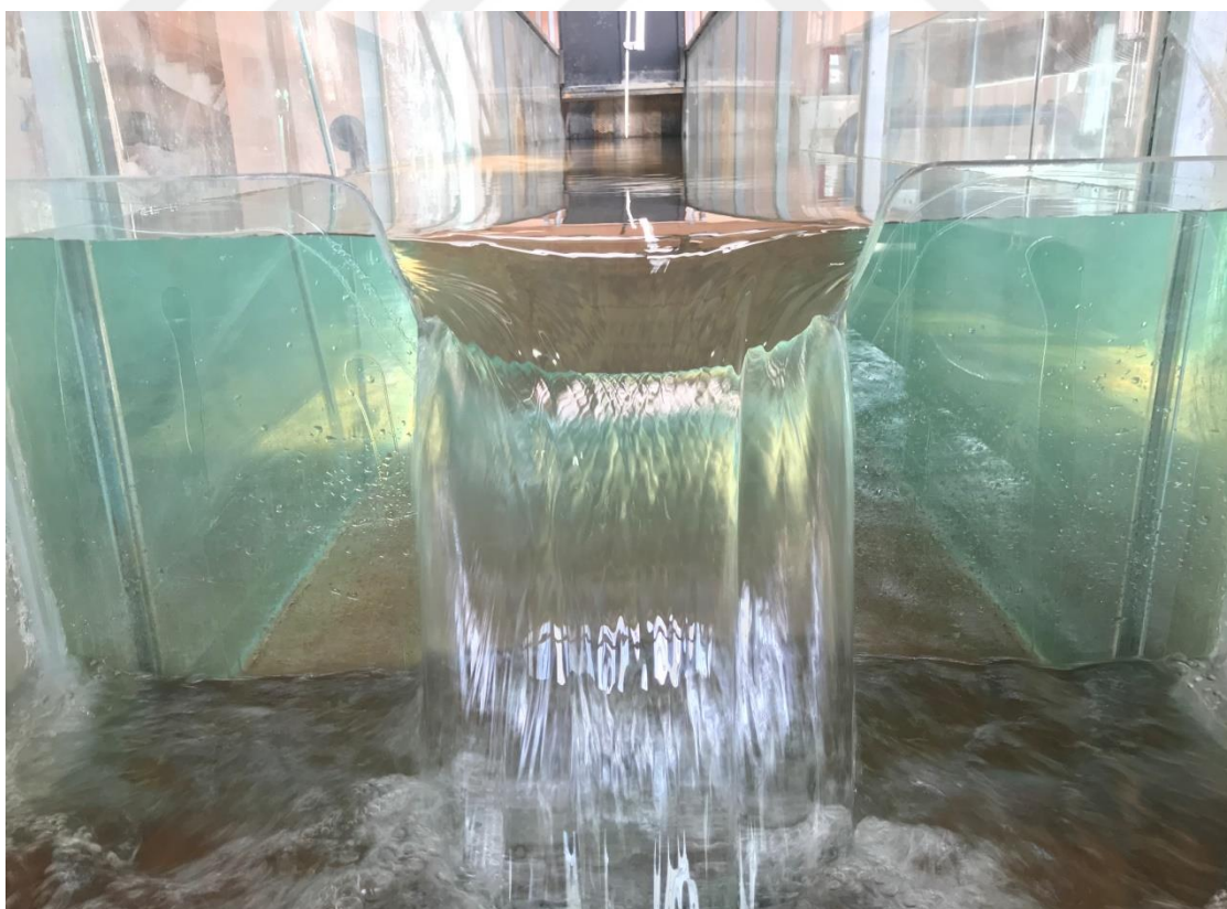
Figure 3.12 Semi-circular weirs with semi-circular edge model with R = 0.15 m during the experiments
