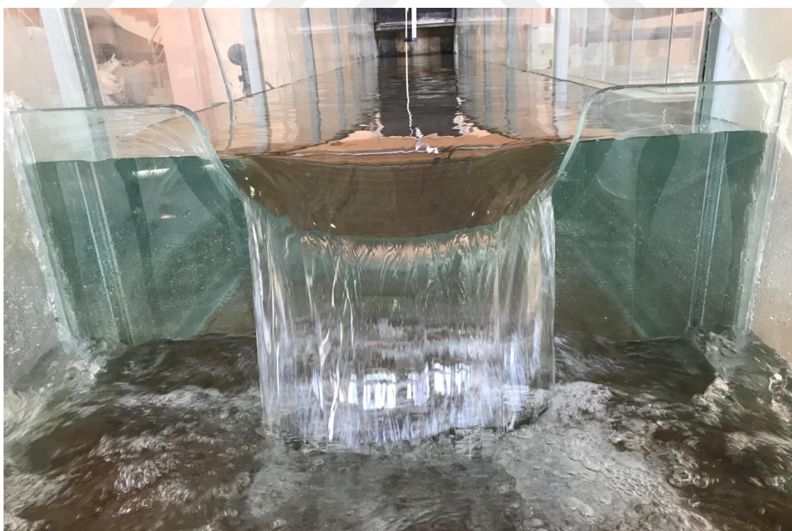
Figure 3.14 Semi-circular weirs with semi-circular edge model with R = 0.20 m during the experiments
