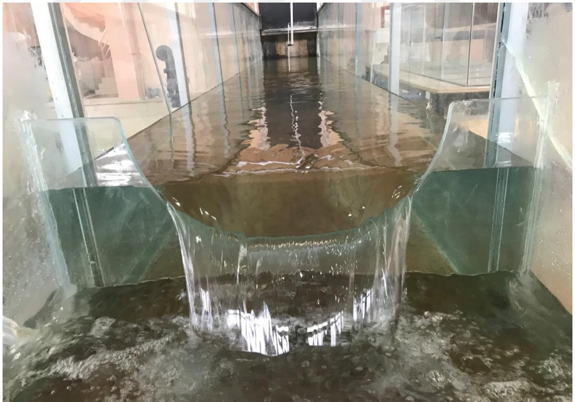
Figure 3.16 Semi-circular weirs with semi-circular edge model with R = 0.25 m during the experiments
