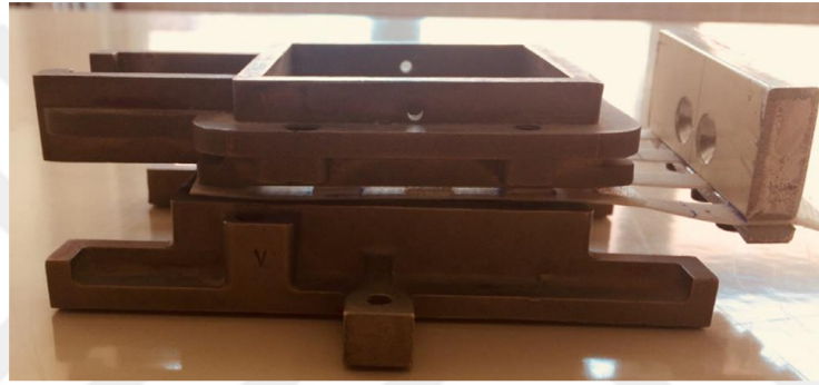
Figure 4.19. Special cap for direct shear test (Altay et al., 2019)
