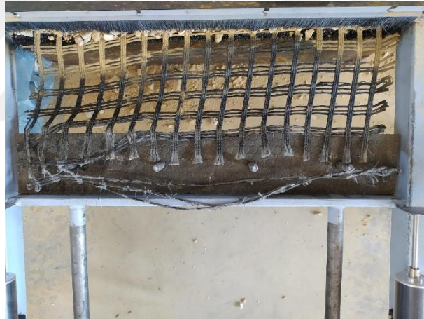
Figure 6.7. Unsuccessful pullout test due to the loosen of bolts
