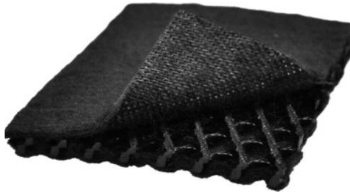
Figure 2.12. Geocomposite material based on geotextile and geonet (Narejo et al., 2013)
