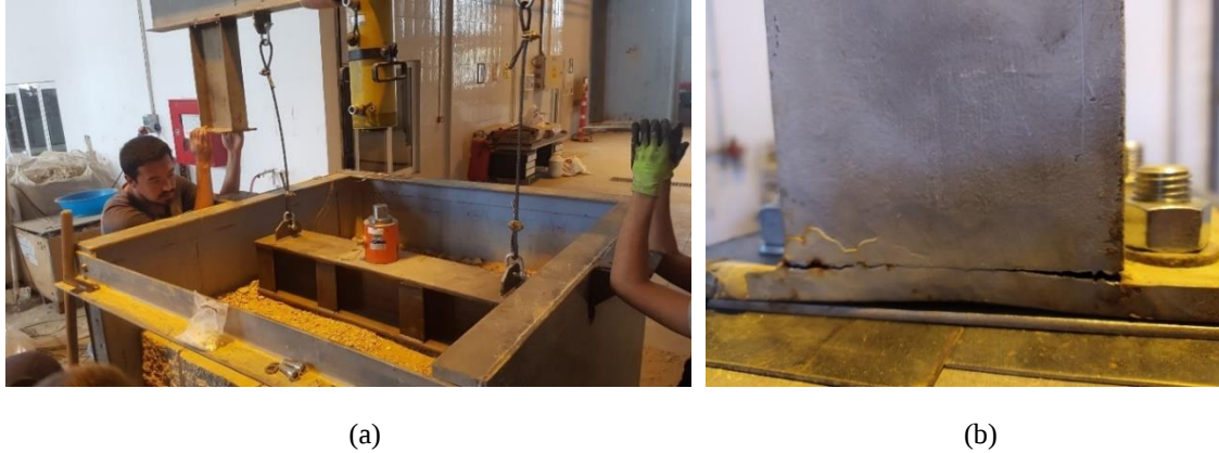
Figure 8.11. a) Placement of the upper part of the experimental setup, and b) Fractures from welding point occurring in the upper part of the experimental setup
