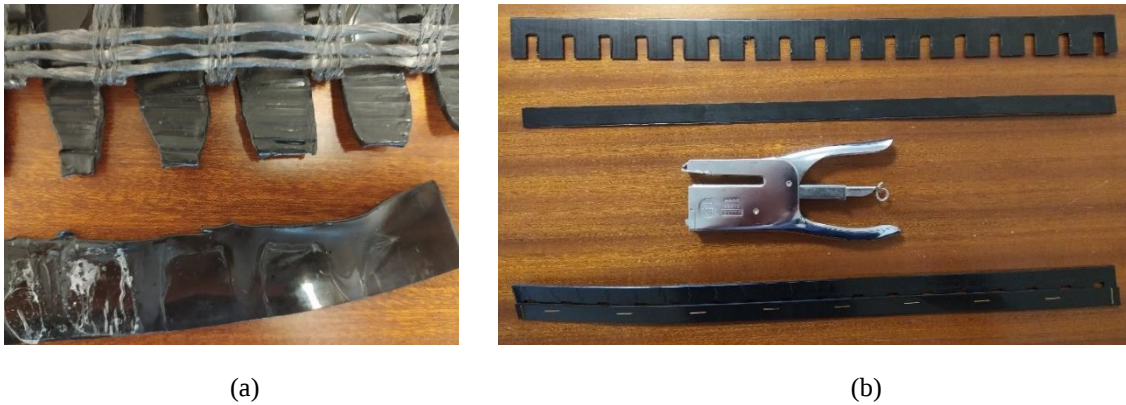
Figure 5.12. a) Attempt to fuse geomembrane pieces by melting with heat, and b) Lower piece, upper piece, and geomembrane joined with staples
