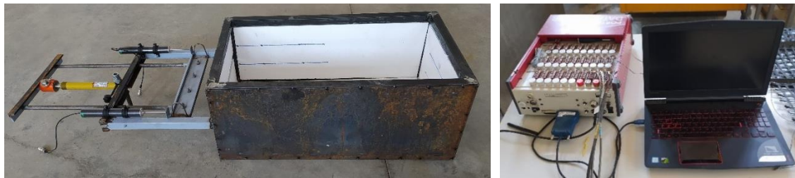
Figure 6.4. a) Pullout test setup, and b) Datalogger
