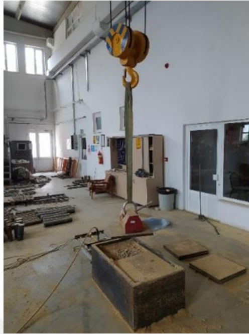
Figure 6.8. The lifting operation of loading plates
