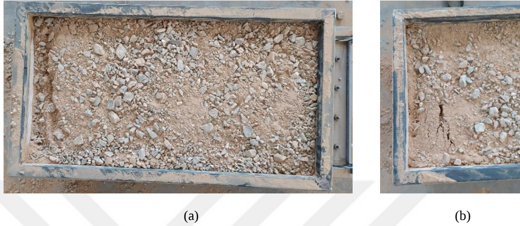
Figure 6.17. The view of the soil surface after pullout test of a) 4T at 6.24 kPa and b) 16T at 8.40 kPa
