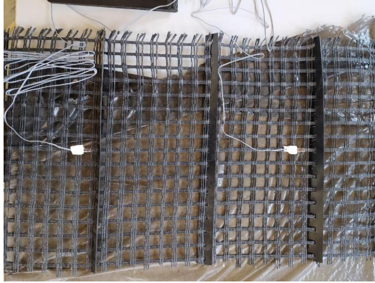
Figure 6.5. The 4T sample with two strain gauges
