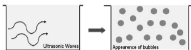
Figure 2.11 Cavitation phenomena in the fluid system (Majid et al., 2015)
