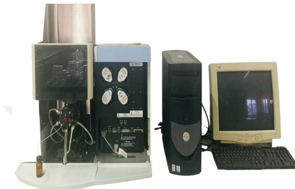
Figure 3.14. Flame atomic absorption spectrometer (FAAS)
