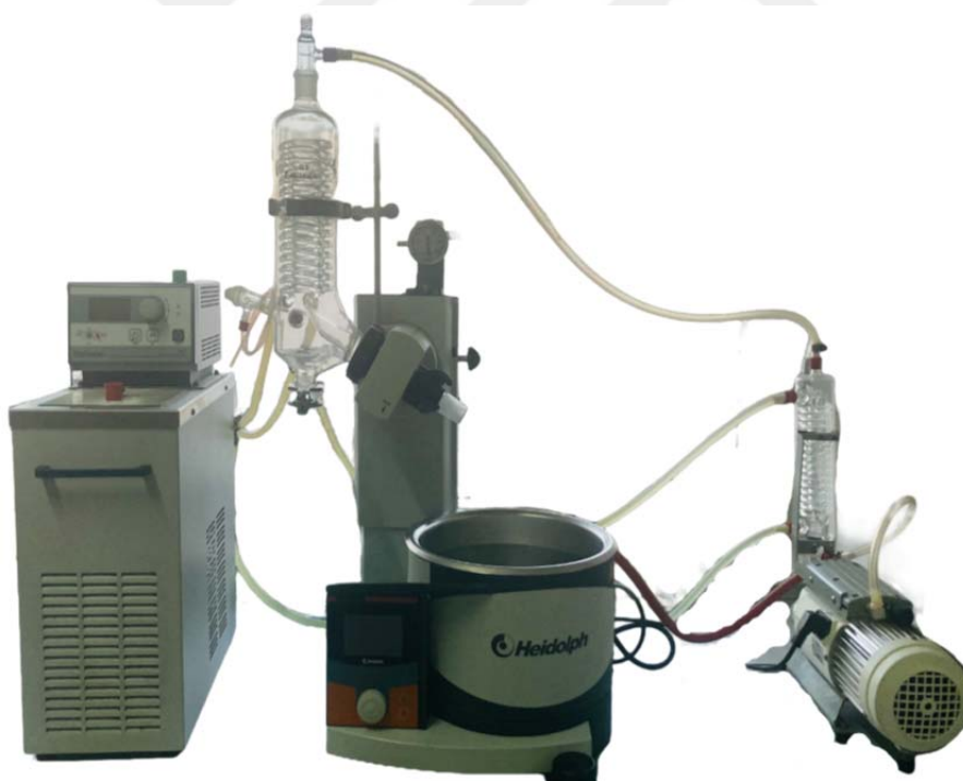
Figure 3.11. Vacuum rotary evaporator (Heidolph, Hei-VAP, Germany)
