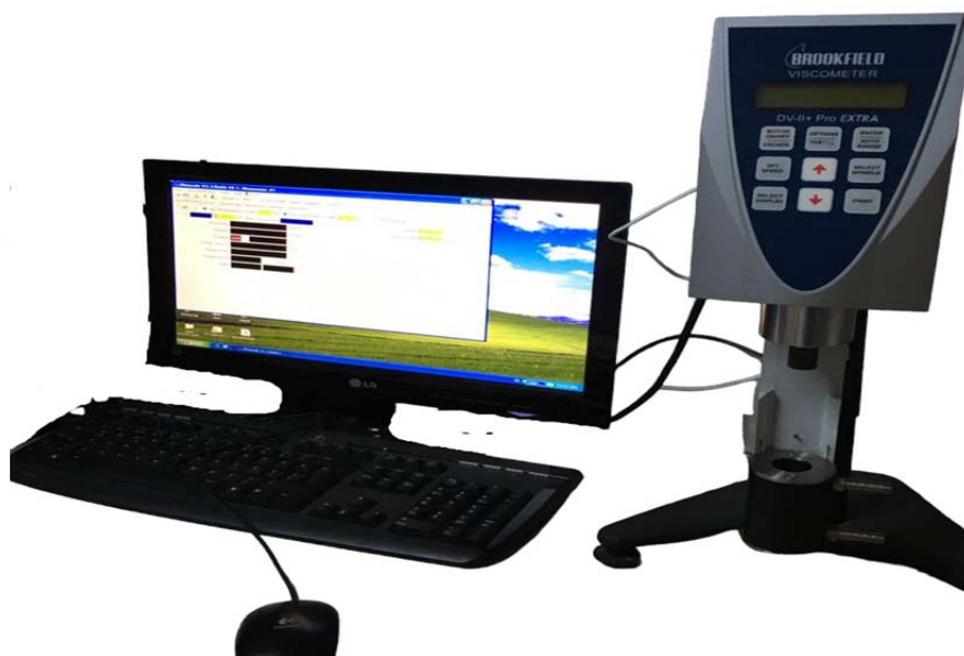
Figure 3.12. DV-II+Pro viscometer (Brookfield)
