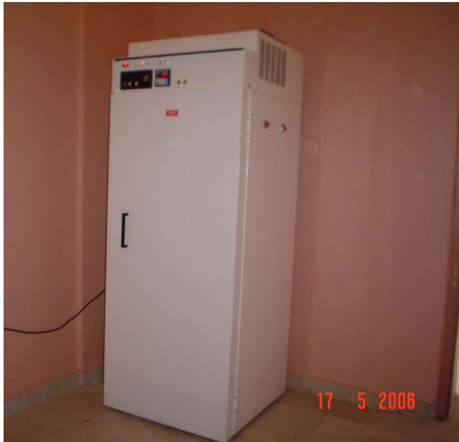
Figure A3 The humidity cabinet for the shrinkage test specimens
