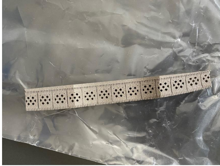
Figure 3.4: Horizontal Sample Side Support Structure
