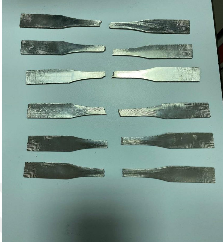
Figure 4.20: Fractured Specimens After Six Tensile Tests
