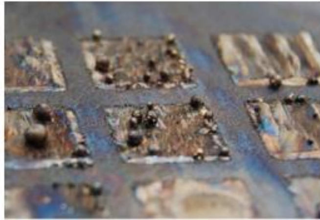
Figure 2.4: Melt ball formation [21]
