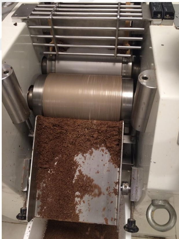
Figure A.11 Refining of chocolate production
