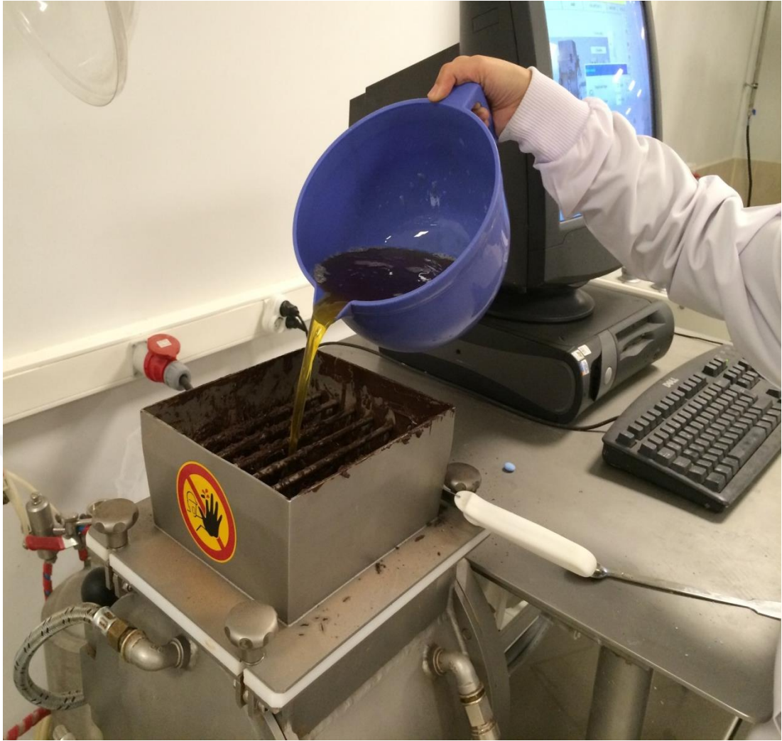
Figure A.12 Conching step of chocolate production
