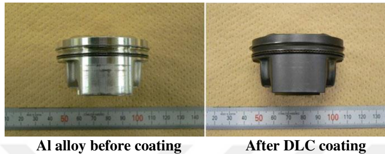
Figure 3.9. DLC-coated aluminum alloy piston
