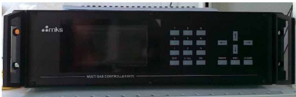
Figure 3.24. Gas Flow-Pressure Control System
