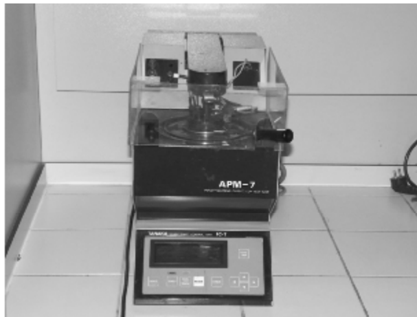
Figure 3.7. Tanaka APM-7 flash point tester
