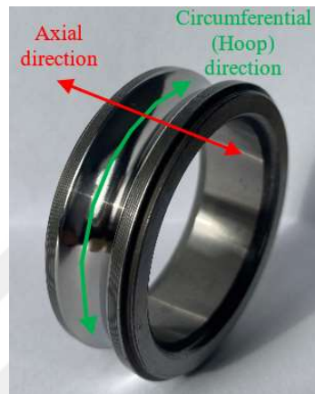
Figure 1.27 The measurement directions of residual stresses for an inner ring
