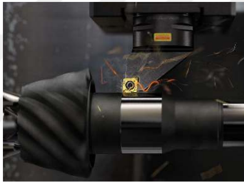
Figure 1.1 A hard turning process [10]
