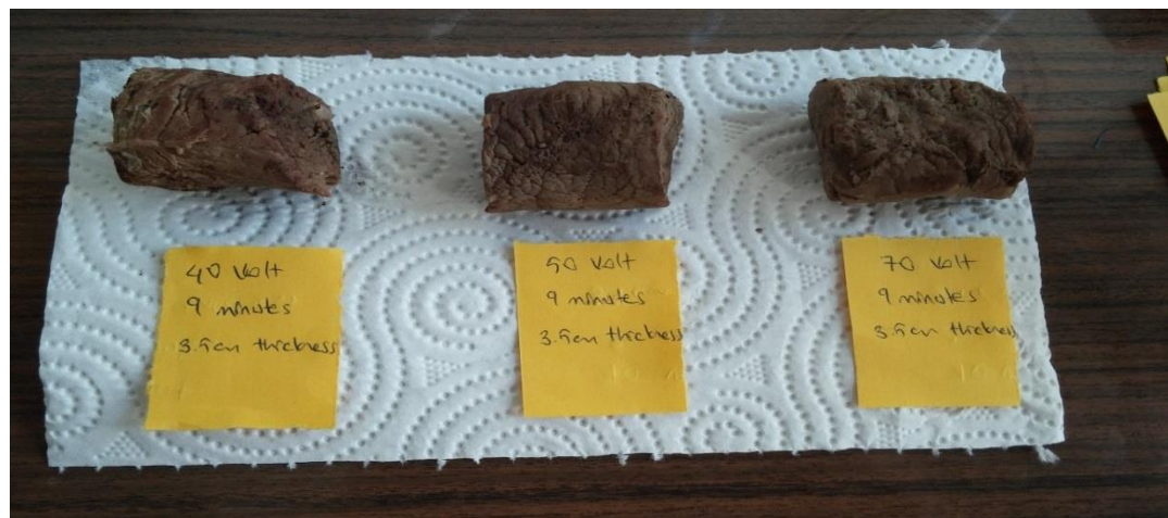
Figure 2.10 Ohmic cooking trials for 40, 50 and 70 V and 9 minutes
