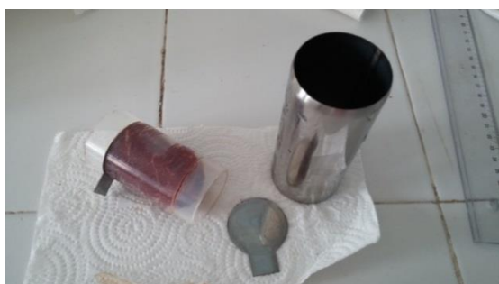
Figure 2.7 Test cell, a meat cutter, 3.5 cm diameter stainless steel electrodes
