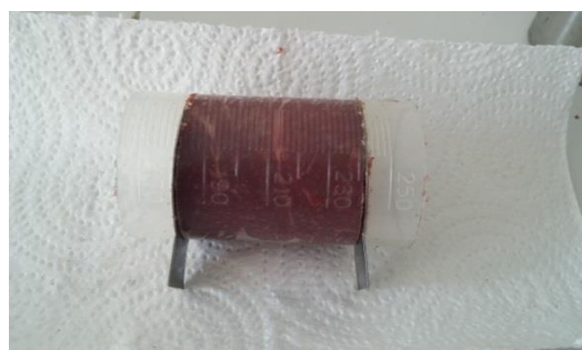
Figure 2.8 Meat inside test cell is ready for ohmic cooking
