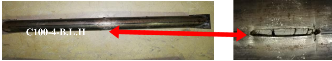
(C) Sample no three C100-4-BLH of the first group failure modes
