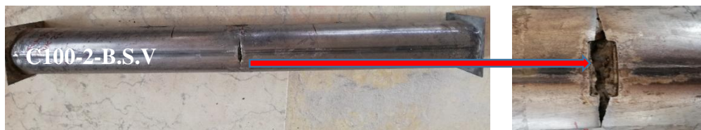
(B) Sample no two C100-2-BSV of the fourth group failure modes
