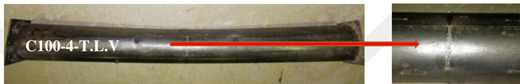
(D) Sample no three C100-4-TLV of the second group failure modes
