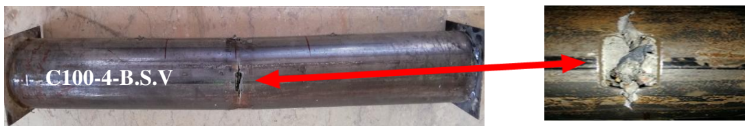
(B) Sample no two C100-4-B.S.V of the first group failure modes
