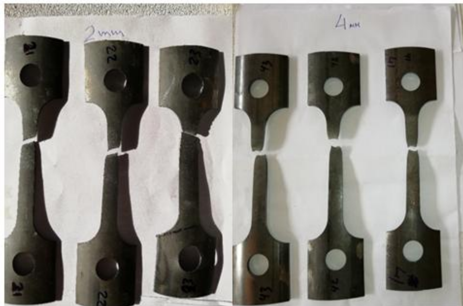
Figure 3.3 Tensile after testing
