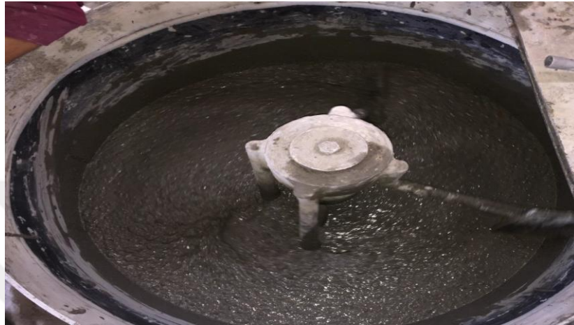
Figure 3.1 Mixing of the SCC
