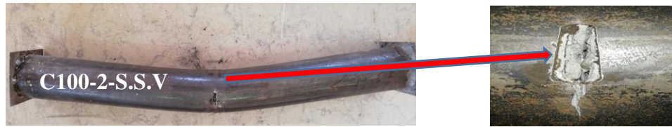
(B) Sample no two C100-2-SSV of the sixth group failure modes
