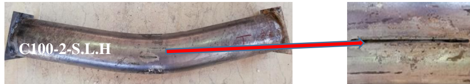
(C) Sample no three C100-2-SLH of the sixth group failure modes
