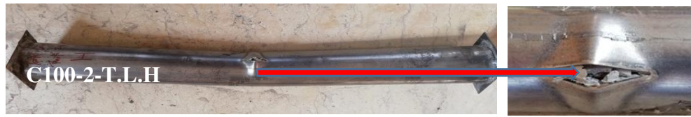
(C) Sample no three C100-2-TLH of the fifth group failure modes
