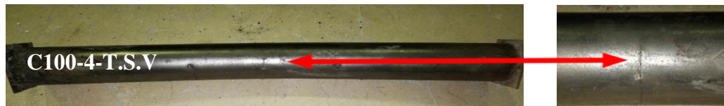
(B) Sample no two C100-4-TSV of the second group failure modes
