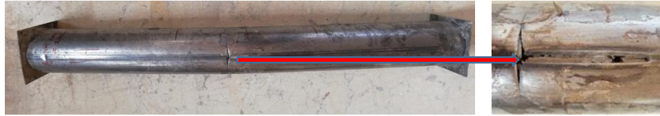
(C) Sample no three C100-2-BSH of the fourth group failure modes after the test
