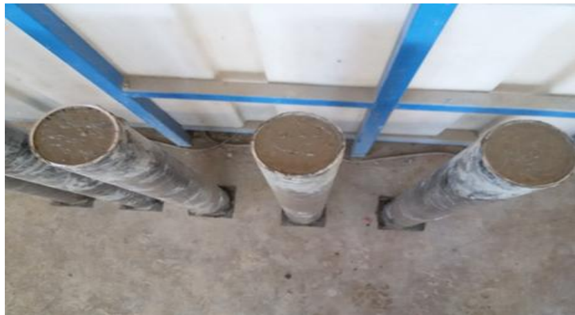
(B) Specimens after casting
