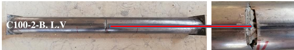
(D) Sample no four C100-2-BLV of the fourth group failure modes
