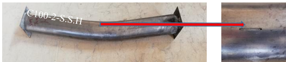
(A) Sample no two C100-2-SSV of the sixth group failure modes
