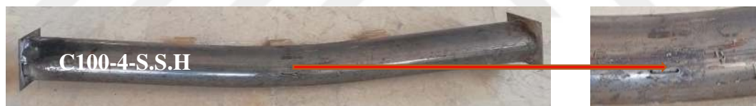
(A) Sample no one C100-4-SSH of the third group failure modes
