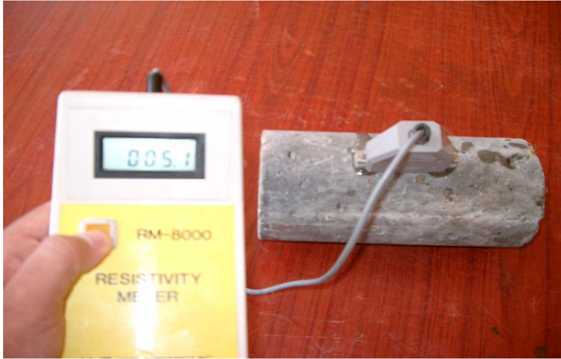
Figure 3.11 Electrical resistivity measurement
