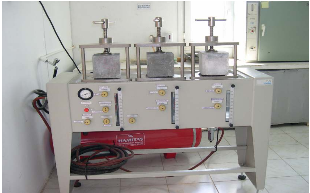
Figure 3.14 Photographic view of water permeability test equipment
