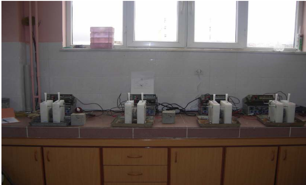
Figure 3.10 Rapid chloride permeability test
