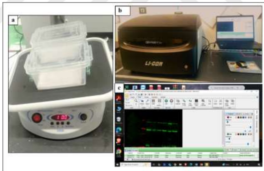
Figure 25. Immunoblotting and imaging. (a) Antibody incubation (primary or secondary). (b) LICOR Odyssey® CLx Imaging System. (c) Protein bands shown in Image Studio® software.
