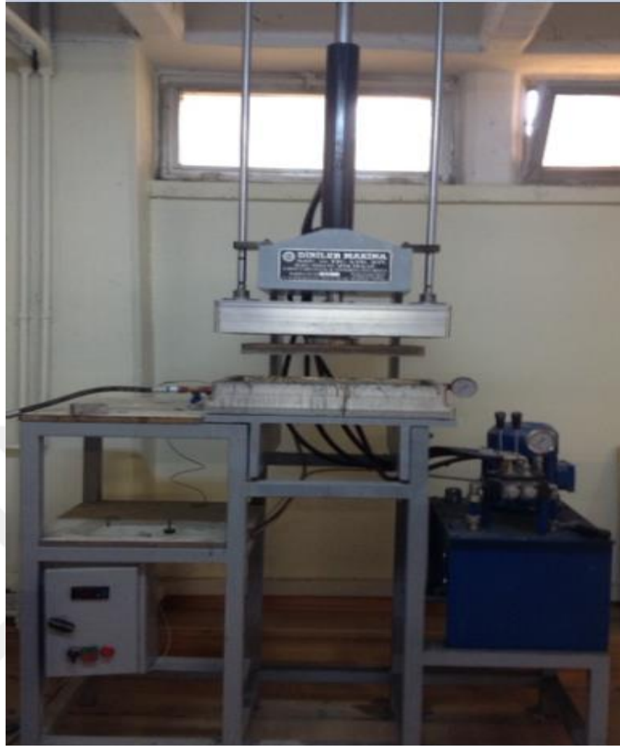
Figure 3.5 composite production unit. (1) Combination of heat, pressure (2) Hydraulic unit.
