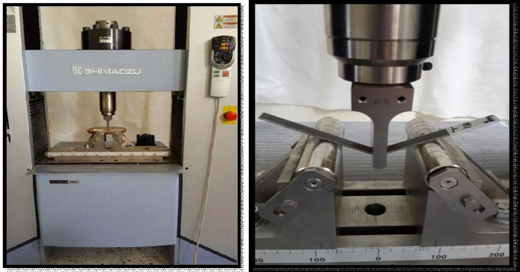
Figure 3.15 (a) Flexural test method, (b) Specimen under test.
