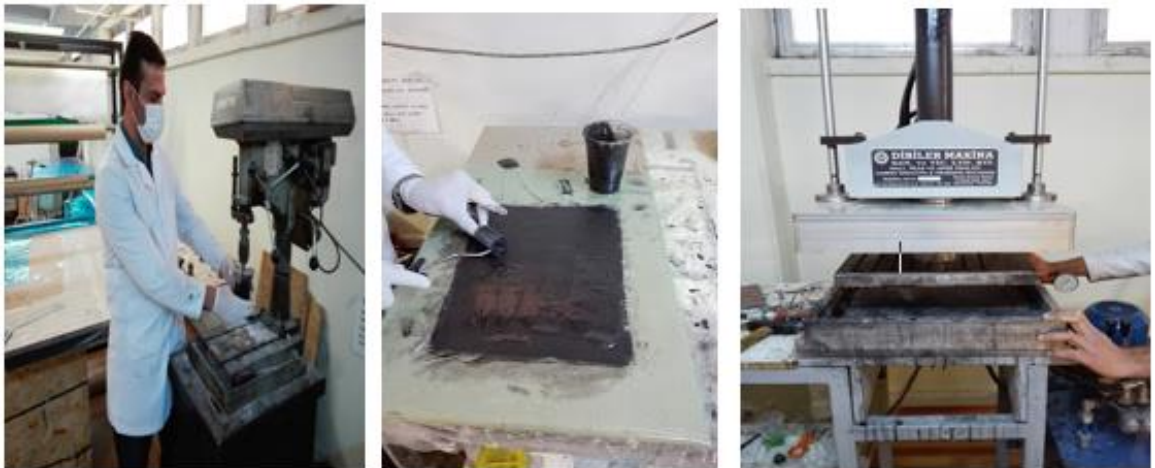
Figure 3.4 Mixing, Laying of nanographene/epoxy resin, Molding
