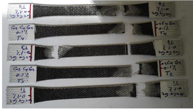
Figure 4.18 Tensile samples after failure of G2C4G2 hybrid composite filled with nanographene
