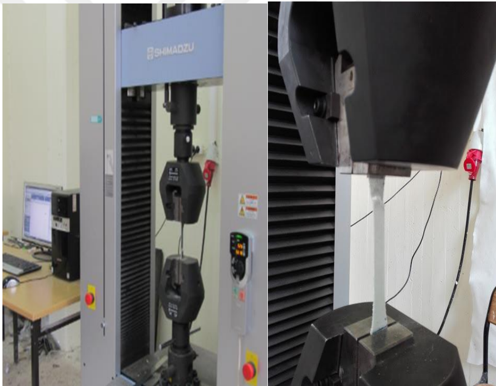
Figure 3.12 Test set-up Shimadzu AG-X series testing machine, specimen under test.
