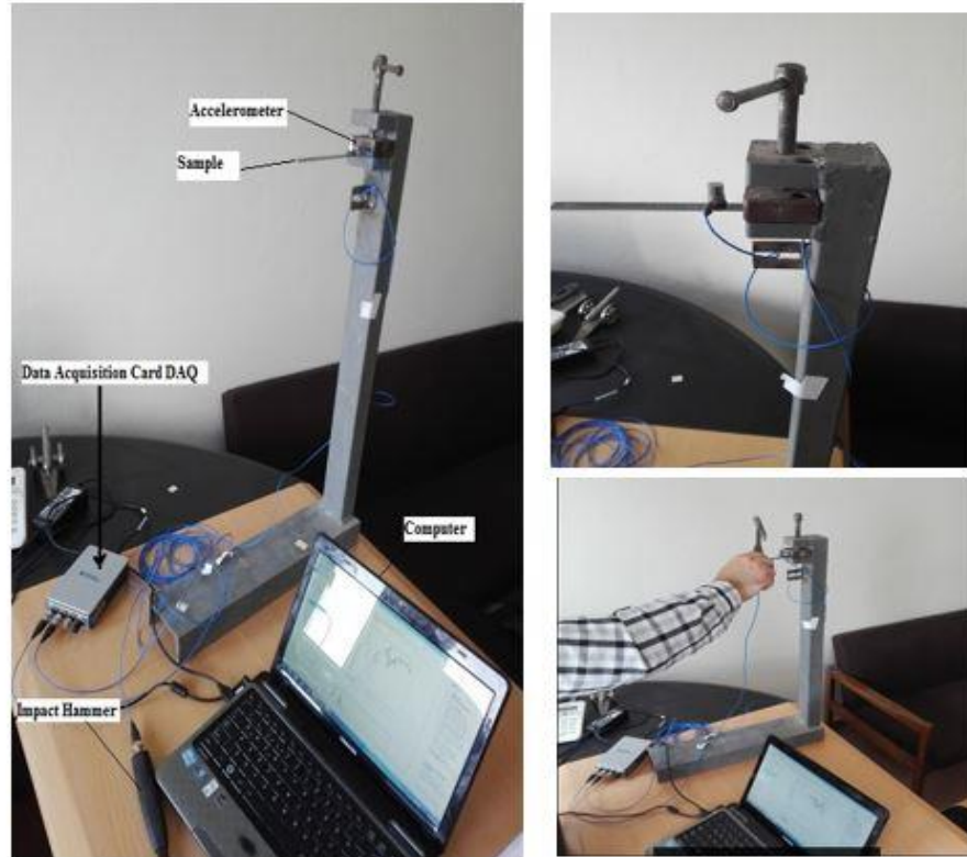
Figure 3.19 Experimental set-up of vibration damping test
