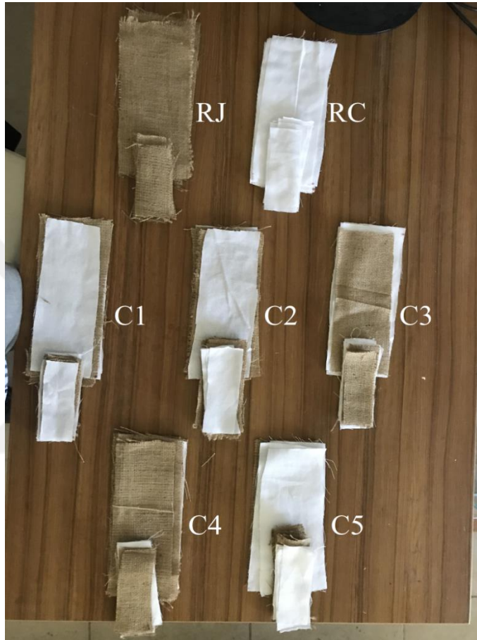
Figure 3.4. The cut fabrics to produce tensile and impact test specimens
