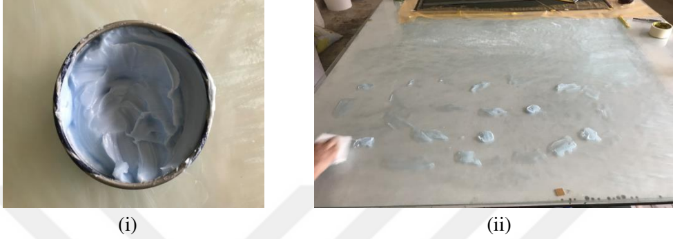
Figure 3.5. (i) Mold release wax (ii) application to the surface
