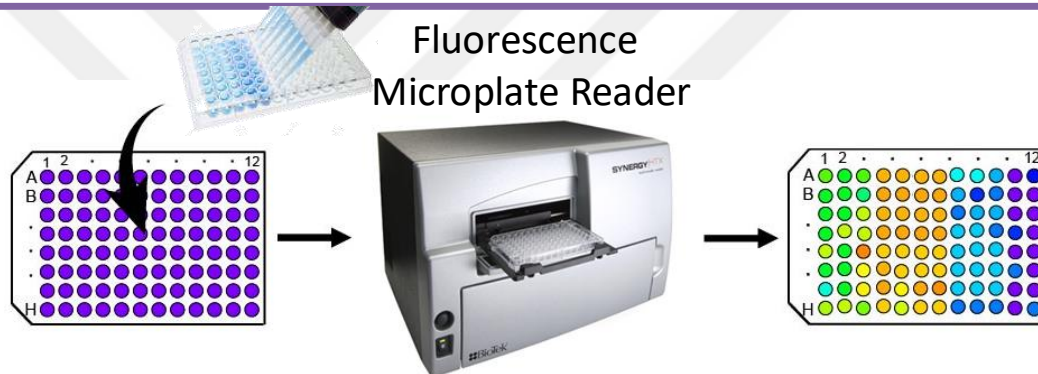
Illustration 4.4 Fluorimetric microplate enzyme assay for measuring extracellular enzymes.
