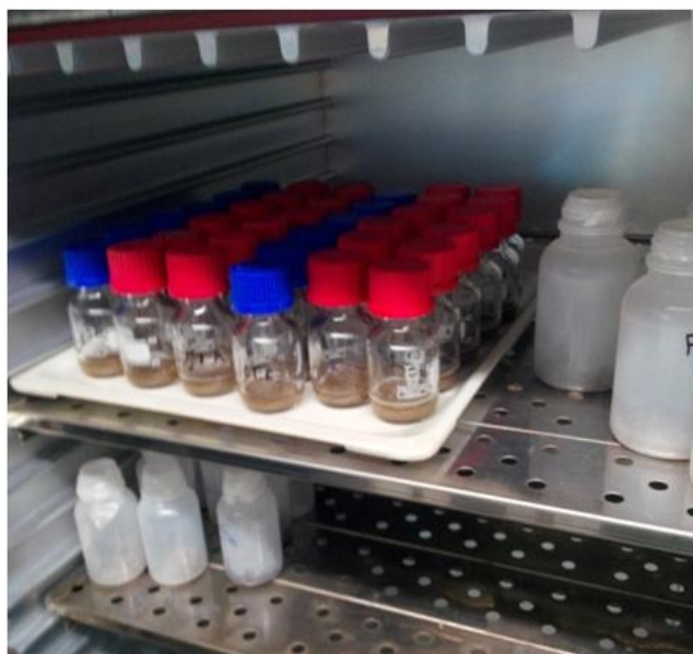
Figure 4.1 Acetone treated soil samples in measure dehydrogenase activity with TTC method.
