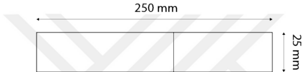
Figure 4.8. Dimensions of Tensile Test Specimen
