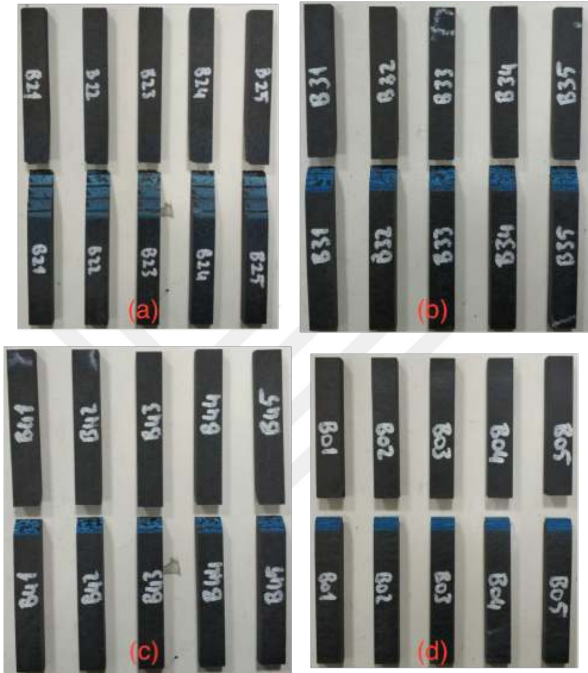
Figure 5.18. Fractured samples repaired with 20° in (a), 30° in (b), 45° in (c) and double scarf in (d) after bending test
