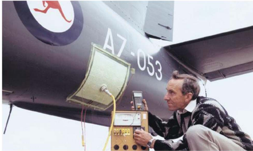
Figure 1.1. Repair of an airframe with a patch [6]
