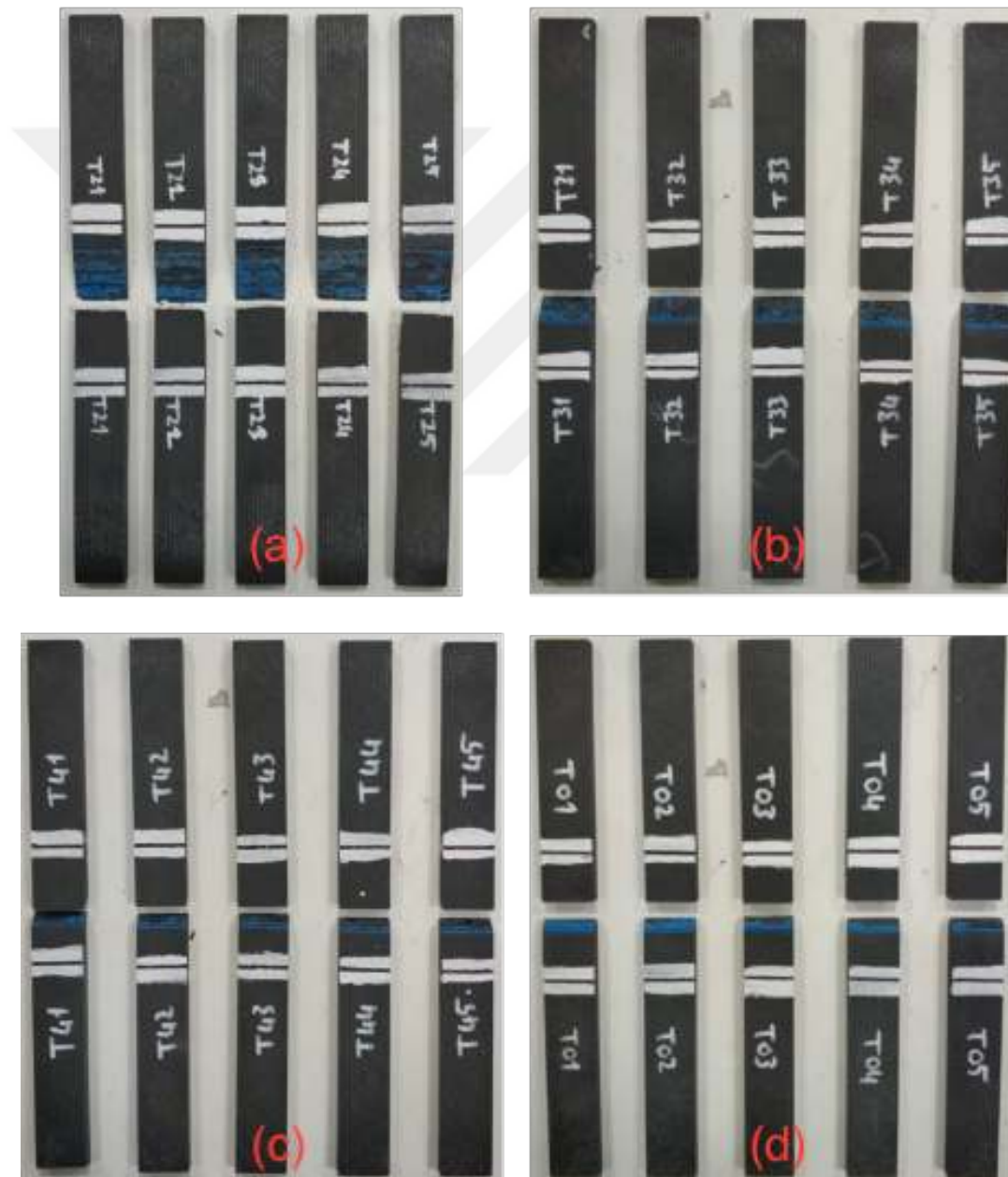
Figure 5.8. Broken specimens repaired with 20° in (a), 30° in (b), 45° in (c) and double scarf in (d) after tensile test
