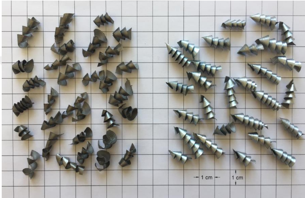
Figure 3.19 Photo of uncoated (left) and coated (right) steel CNC milling waste (type A).
