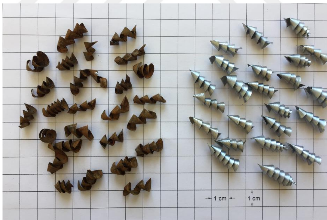
Figure 4.19 Photo of uncoated (left side) and coated (right side) steel CNC milling waste after immersion in tap water for 72 hours.
