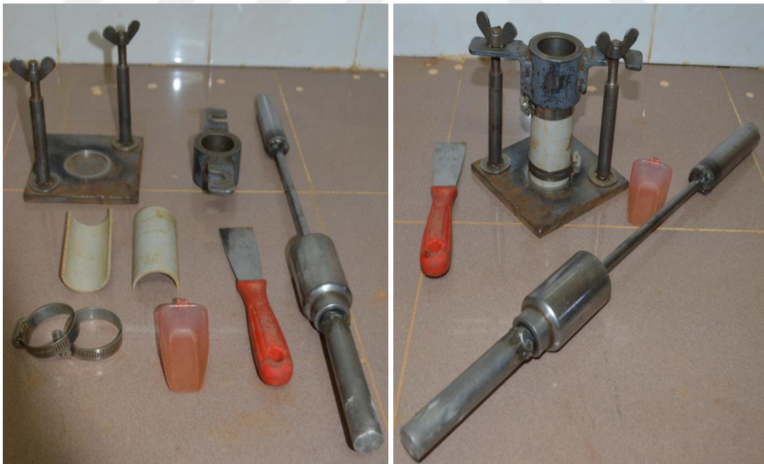
Figure 3.8 The plastic split mold and the compaction hammer for the UCS samples preparation.
