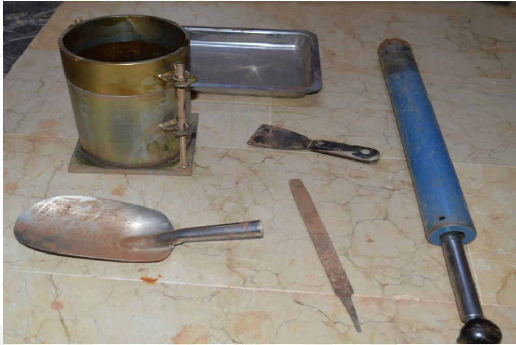
Figure 3.10 The mold and the compaction hammer for the CBR samples preparation.
