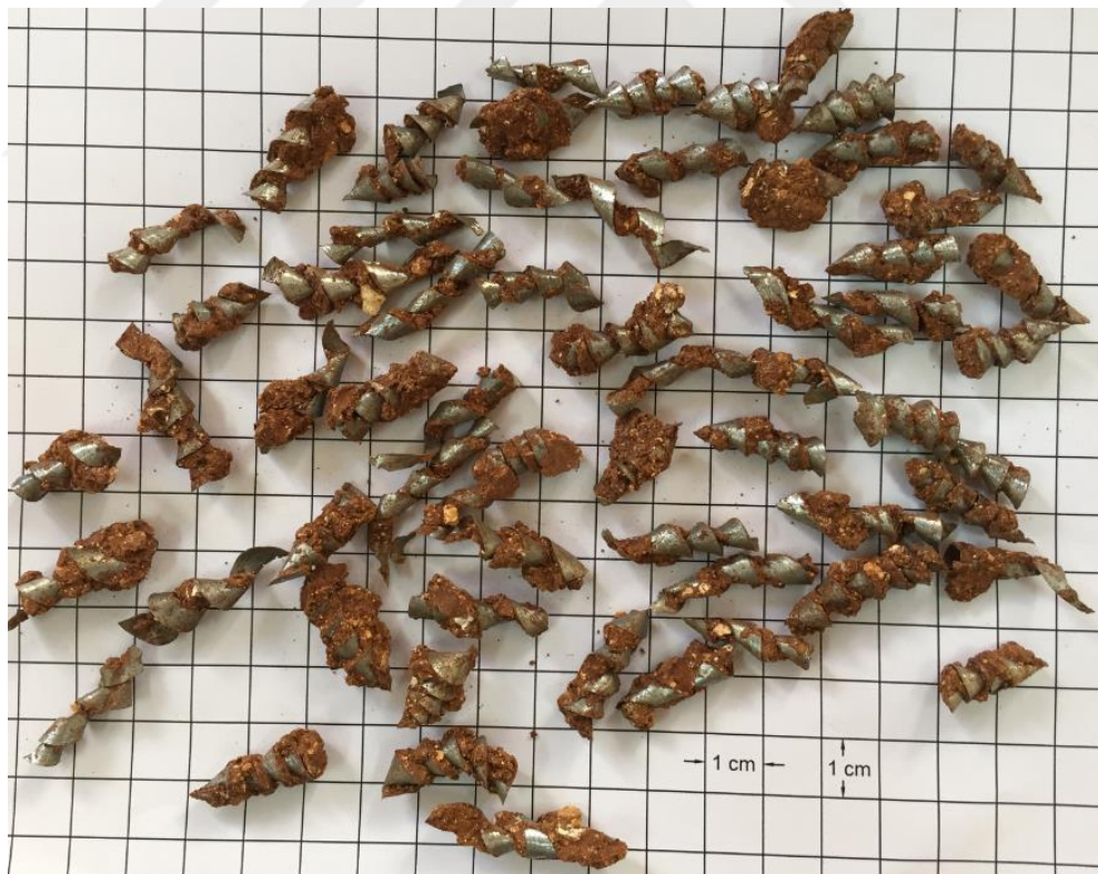
Figure 4.15 Particle of soil with the particle of steel CNC milling waste.
