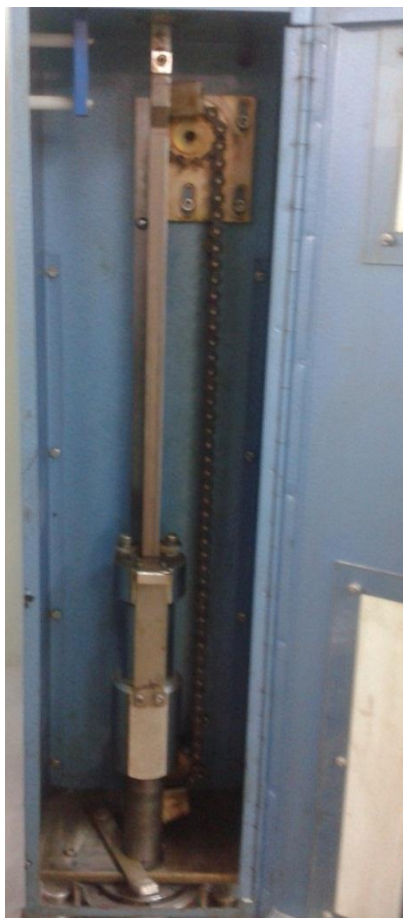
Figure 4.13 Automatic Marshall compactor
