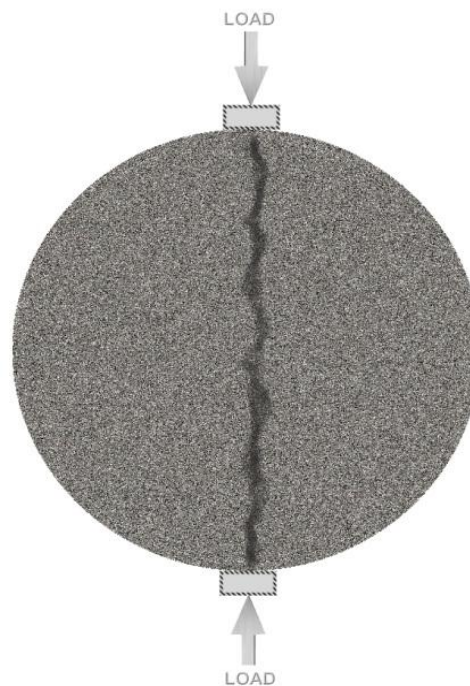
Figure 4.16 A possible crack pattern for IDT test
