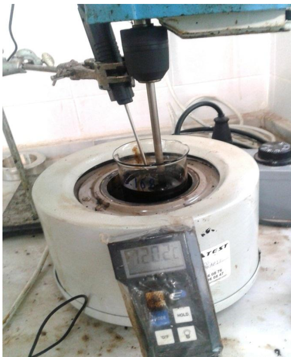
Figure 4.6 Production of WMA bitumens
