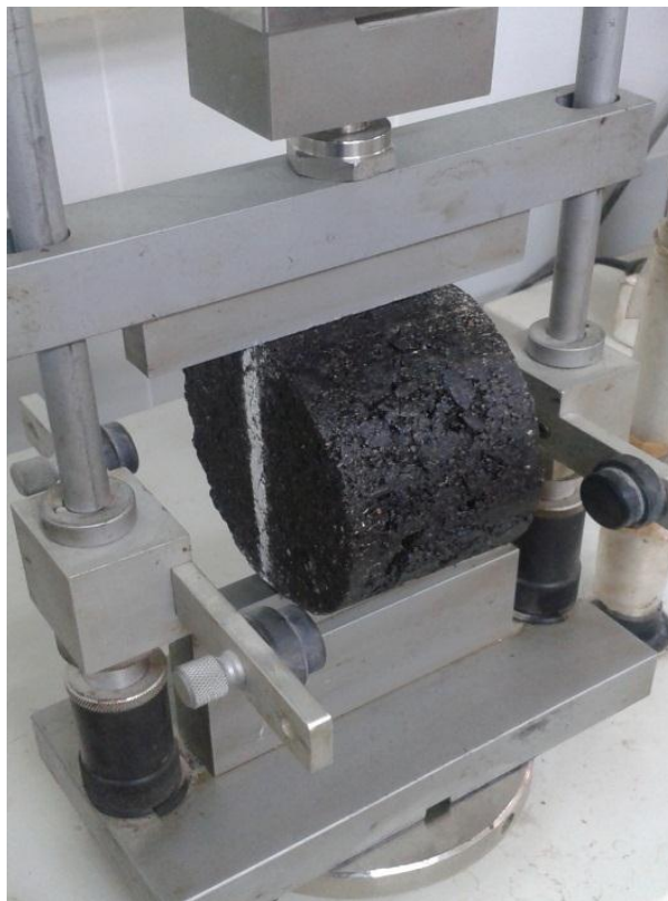
Figure 4.17 Marshall specimen ready for IDT test
