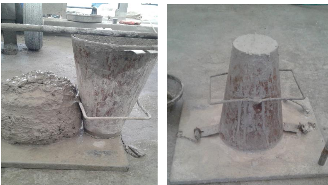
Figure 3.7: Slump Test for Workability
