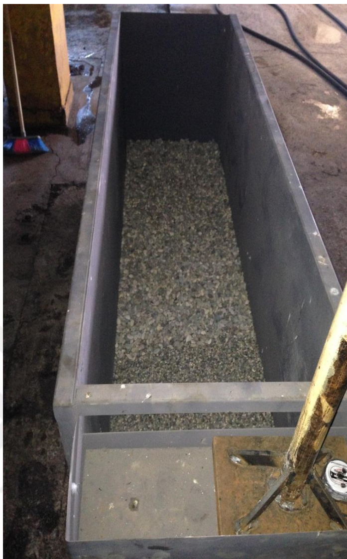
Figure 3.7 Gravel used for filtration
