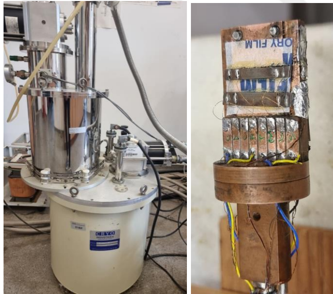
Figure 5.3. cryostat system for characterization of superconducting properties of samples.
