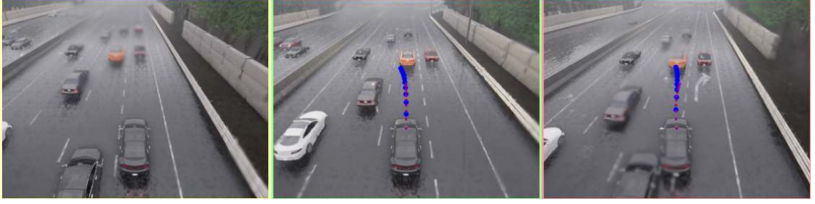
Figure 4.5: Lane Change without Forecasting. Left: The initial state of the scene, where the ego vehicle is tasked with switching to the left lane. Middle: The Async Model successfully executes the lane change while avoiding collisions by leveraging forecasting. Right: The version without forecasting ( A ) fails to anticipate the future position of the vehicle behind, resulting in a rear-end collision. The predicted action for each model is overlaid on the image, with waypoints shown in blue and the path in red.
