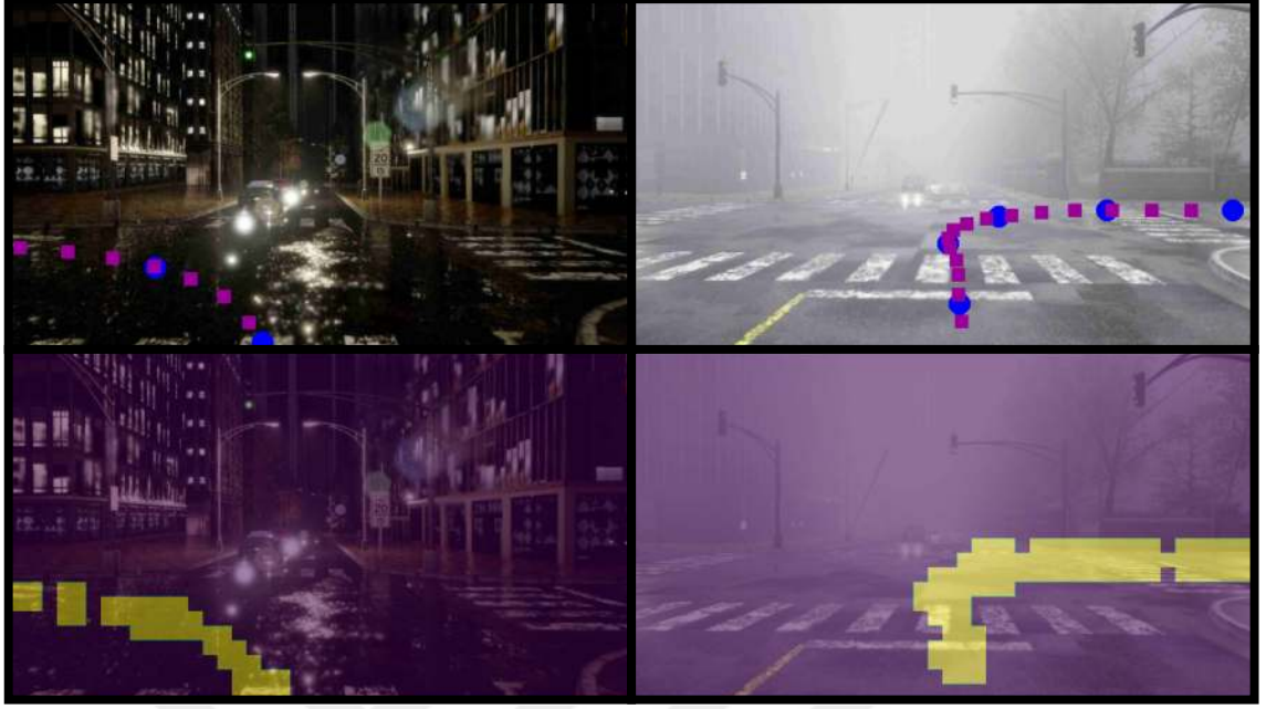
Figure 4.3: Action Mask. In the top row, we show two examples of the RGB image with the path (purple) and waypoints (blue) projected onto it. Patches containing a path or waypoint are marked as 1 (yellow), and all other patches are marked as 0 (purple), creating the binary mask, overlaid on the image below for visualization.
