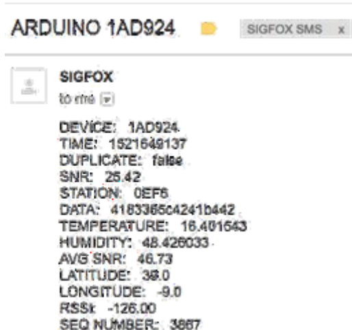
Figure 4.5: Example of an email received using a Sigfox data callback.
