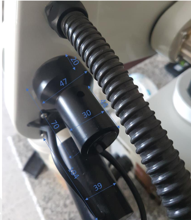
Figure 2.11 Back view measurements between third and fourth actuator from the base (Personal archive, 2020)
