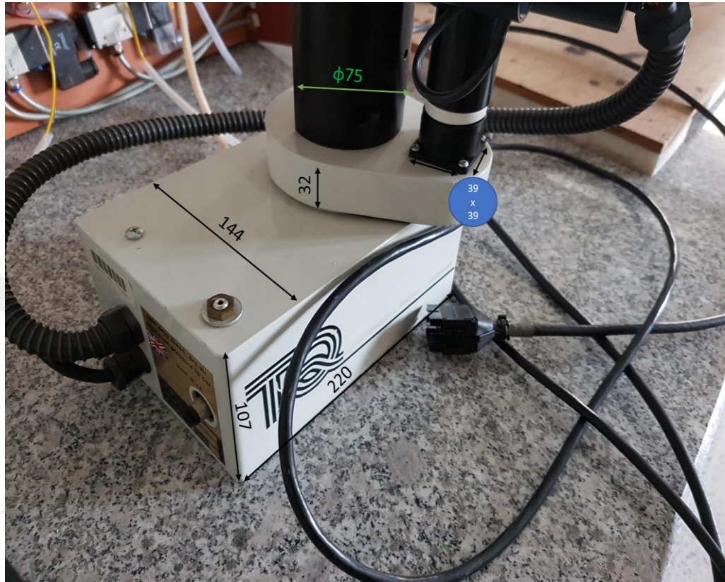
Figure 2.5 Measurements illustrated at the base of TQ MA 2000 (Personal archive, 2020)
