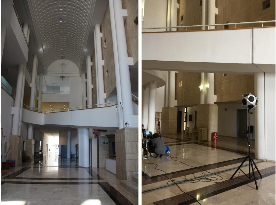
Fig. 6. Interior views of FF atrium, (left) the main atrium space showing barrel-vault ceiling, (right) the offices at the right side of the atrium under the bridge during the field test
