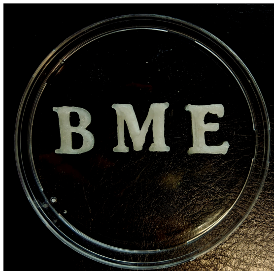
Figure 3.1 Preliminary Printing of MC-Gelatin Hydrogel.
