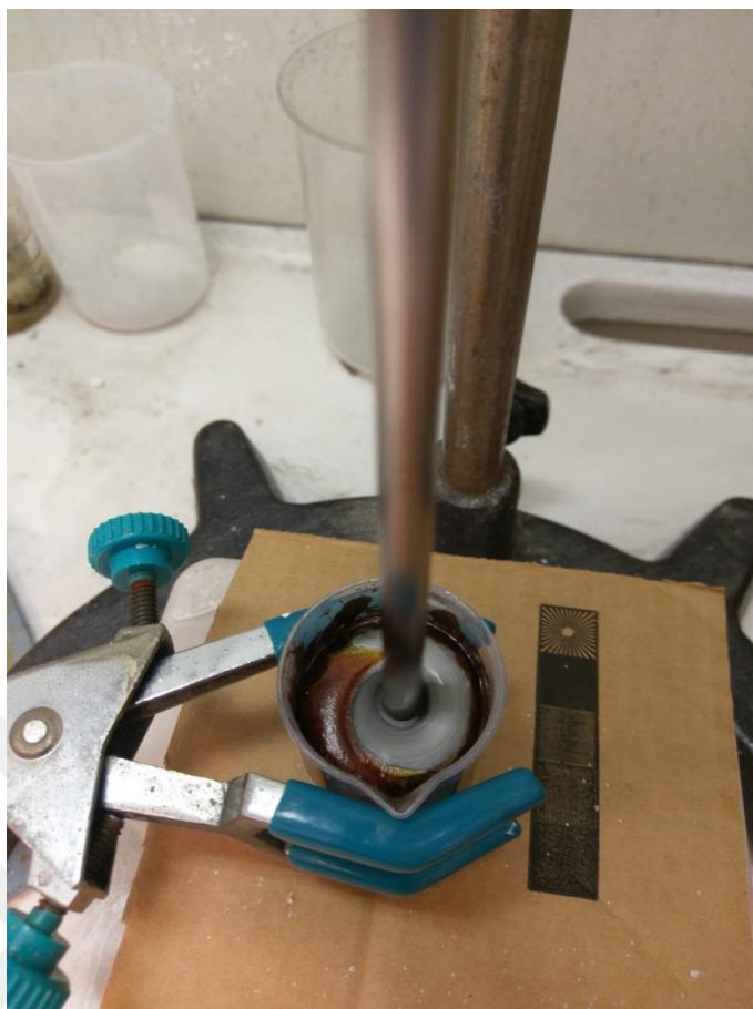
Figure 9 Copolymer and iron flake suspension mixed with a mechanical stirrer
