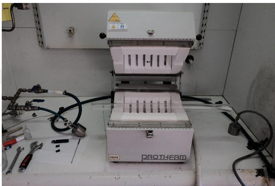
Figure 6 Tube Furnace used in the nitridation process
