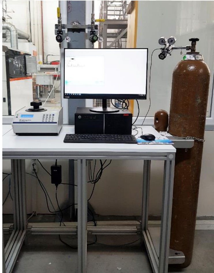
Şekil 3.26. Micromeritics marka AccuPyc II 1340 model gaz piknometresi
