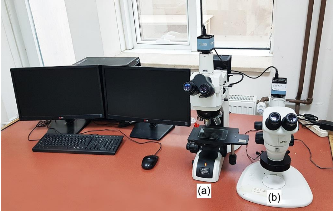
Şekil 3.40. (a) Nikon Marka Eclipse LV150N Model Optik Mikroskop (b) Nikon Marka SMZ 745T Model Stereo Mikroskop
