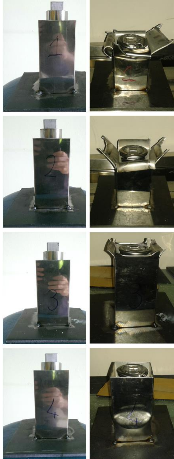
Figure 3.17 : The systems having from in to out: square, circular and square St AISI 304 tubes.
