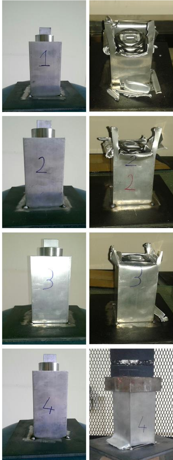
Figure 3.11 : The systems having from in to out: square St AISI 304, circular St AISI 304, square St AISI 304 tubes
