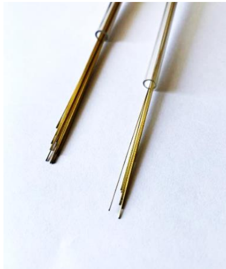
Figure 4.3 Ø500µm and Ø400µm electrodes
