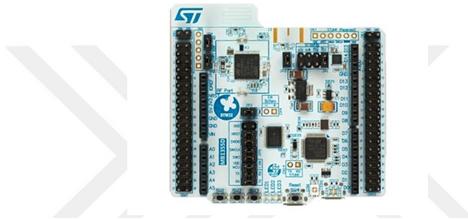
Figure 3.2 : STM32 Nucleo-64 development board with STM32WB55RG MCU
