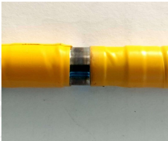
Figure 3.2 Electropolished TG-2 sample at 20^\circ\text{C} , 44 \text{ A/dm}^2 , 3 min. conditions
