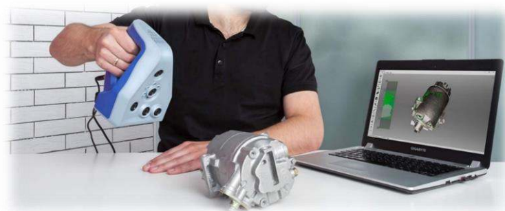
Figure 4.21. Hand-held portable 3-D scanners for CAD users.
