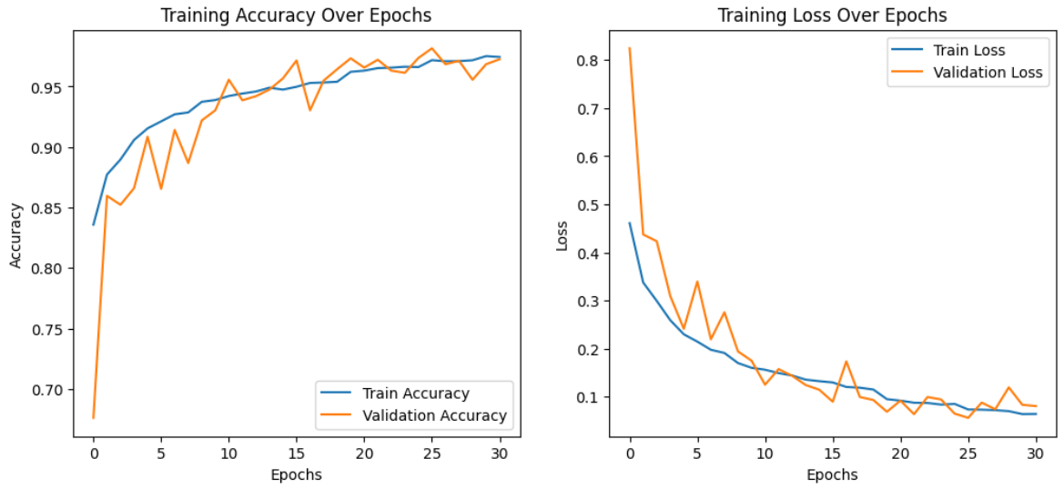
FIGURE 4.3 – FCN model training and validation accuracy/loss over epochs.
