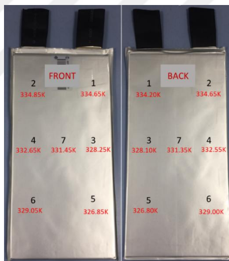
Figure 4.6. Observation of temperature distribution at 5C and 30°C
