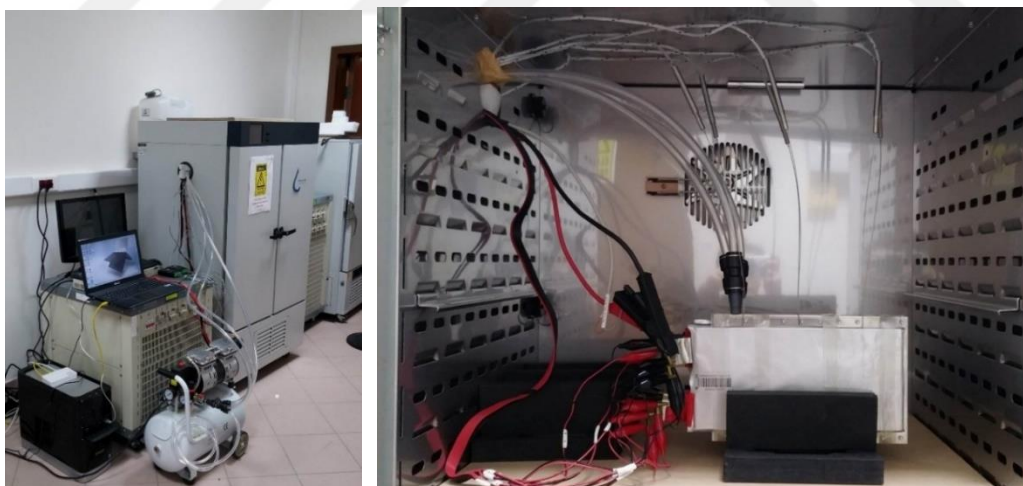
Figure 6.8. Schematic of experimental set up for battery module thermal management.
