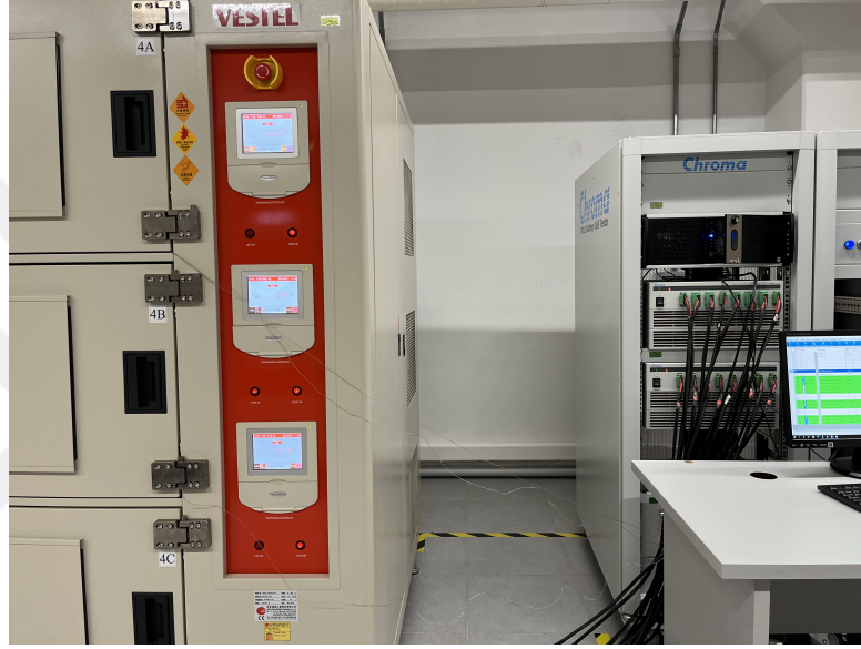
Figure 8: Continuous charging at constant voltage (cells) Test Setup
