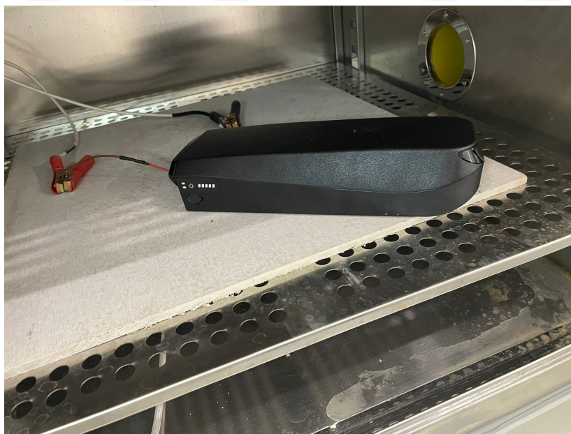
Figure 12: External Short Circuit Test Setup & Exproof chamber
