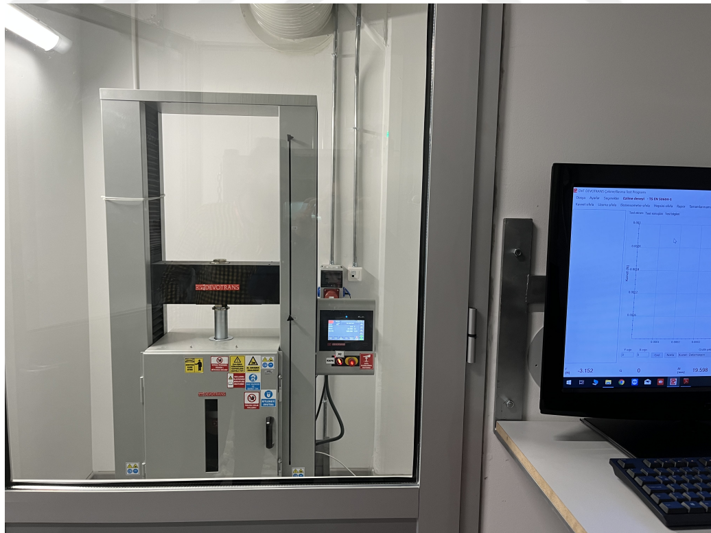
Figure 1: Crush Test Setup & Control Panel
