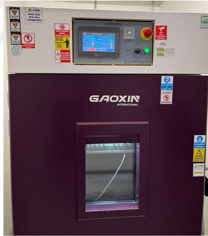
Figure 24: External Short Circuit Chamber Test Setup
