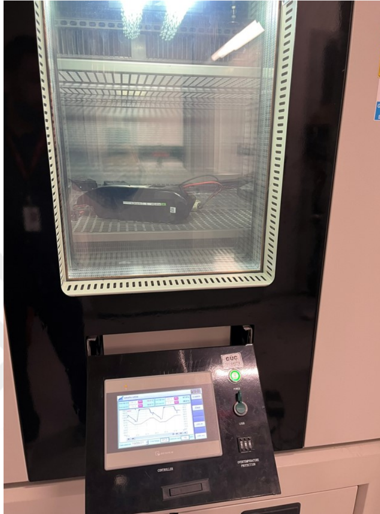
Figure 29: Dewing Test Setup
