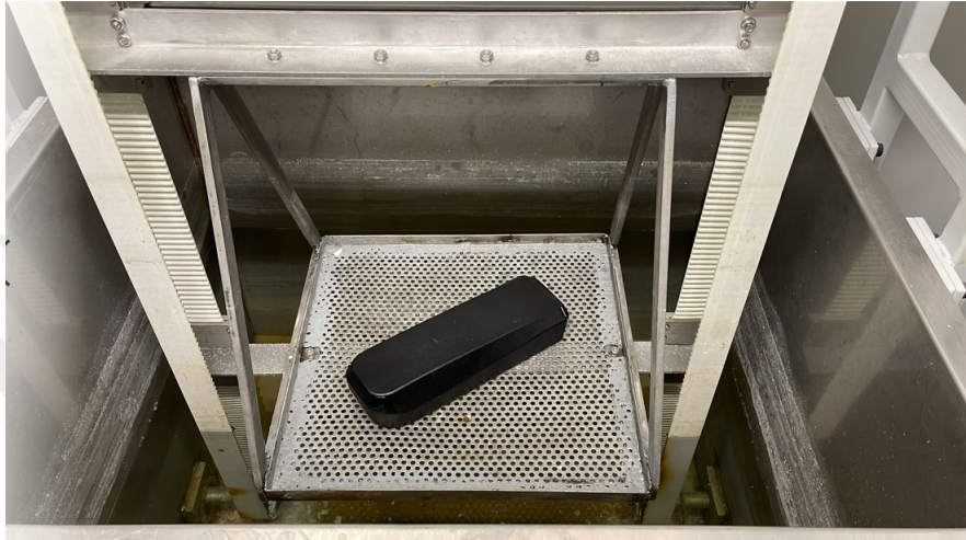
Figure 32: Water Immersion Test Setup
