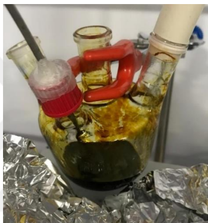
Figure 3.3 Synthesis of the suspension of Ag NPs whose color is reddish brown
