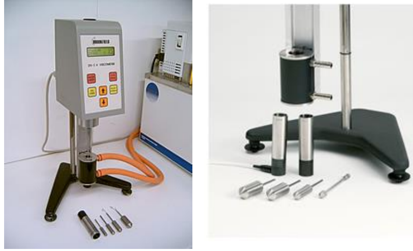
Şekil 7. 12. Brookfield DV-III Viskozimetre (Can-Am Instruments Ltd, 2014)
