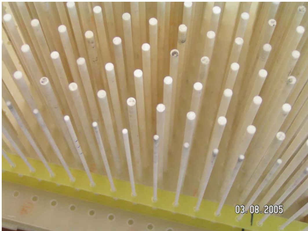
Figure 3.4: The photonic crystal structure that we used in the study of surface modes.
