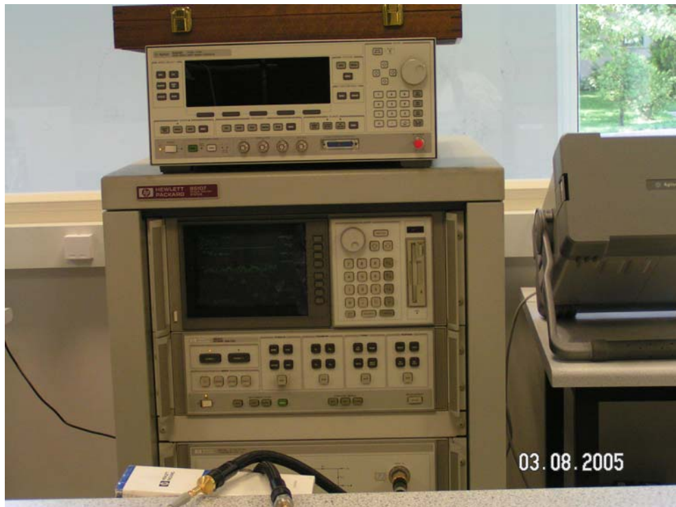
Figure 2.8: The vector network analyzer: HP8510C.
