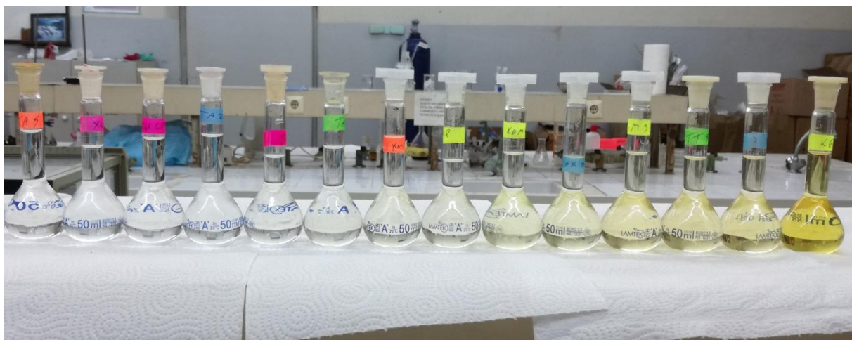
Figure 3.7. Soil Samples After Wet Digestion
