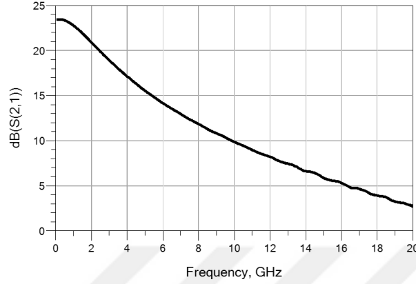
Figure 2.9: Measured S_{21} of a typical 8 \times 100 \mu m device in dB scale on a frequency range of 0.4 GHz to 20.0 GHz.
