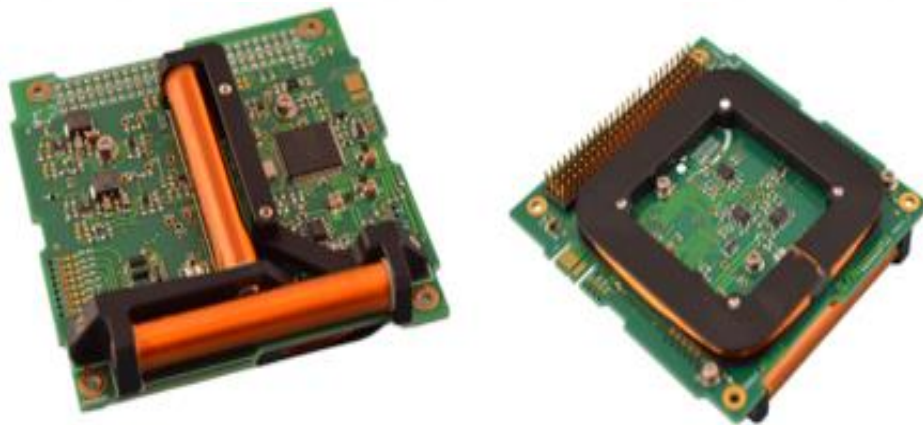
Figure 6: Three actuators; two torque rods and one air core torque. [13]
