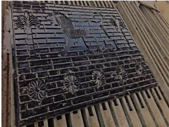
Figure 42. Sample of several mold of fiberglass
